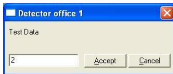
This tool is very useful to test the communication in the *ESSER* panel from the *Modbus* side and vice versa.
