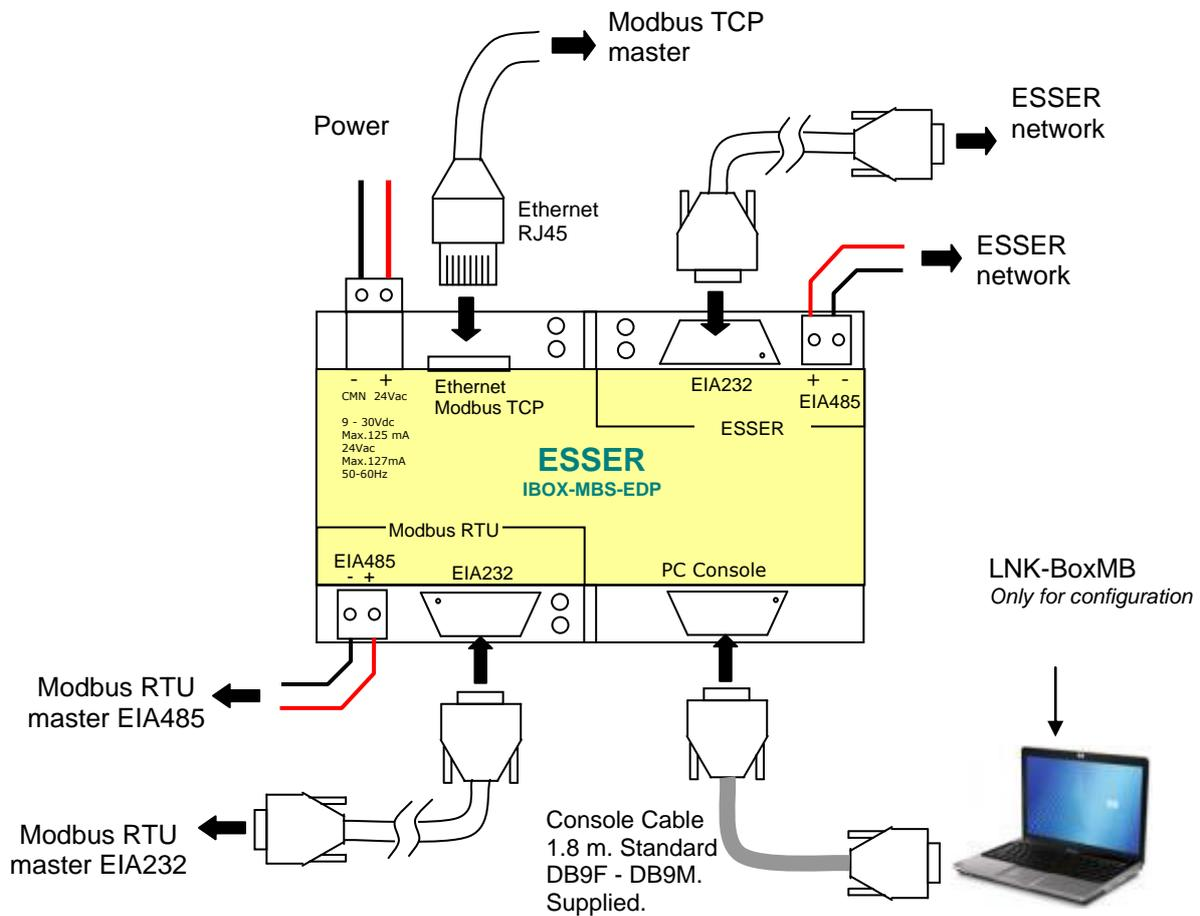
Only one of the ESSER ports of the interface (EIA232 or EIA485) can be used simultaneously, the port to use must be configured within LNK-BoxMB software.
