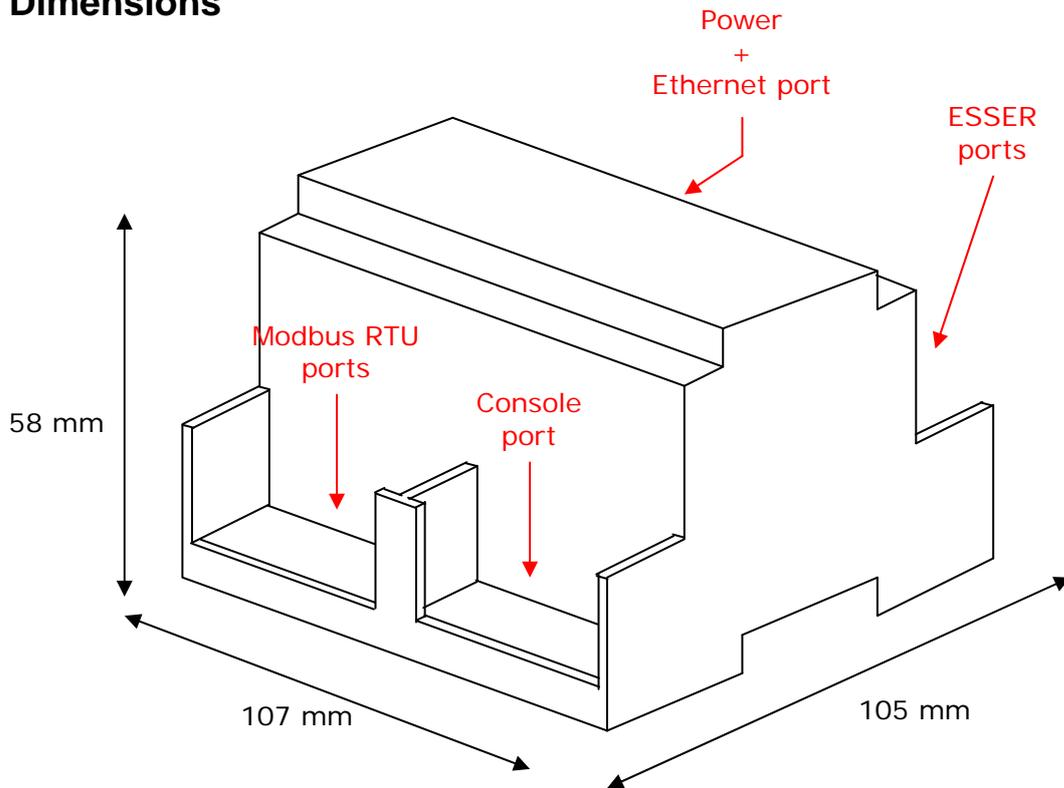
Recommended available space for its installation into a cabinet (wall or DIN rail mounting), with space enough for external connections:
