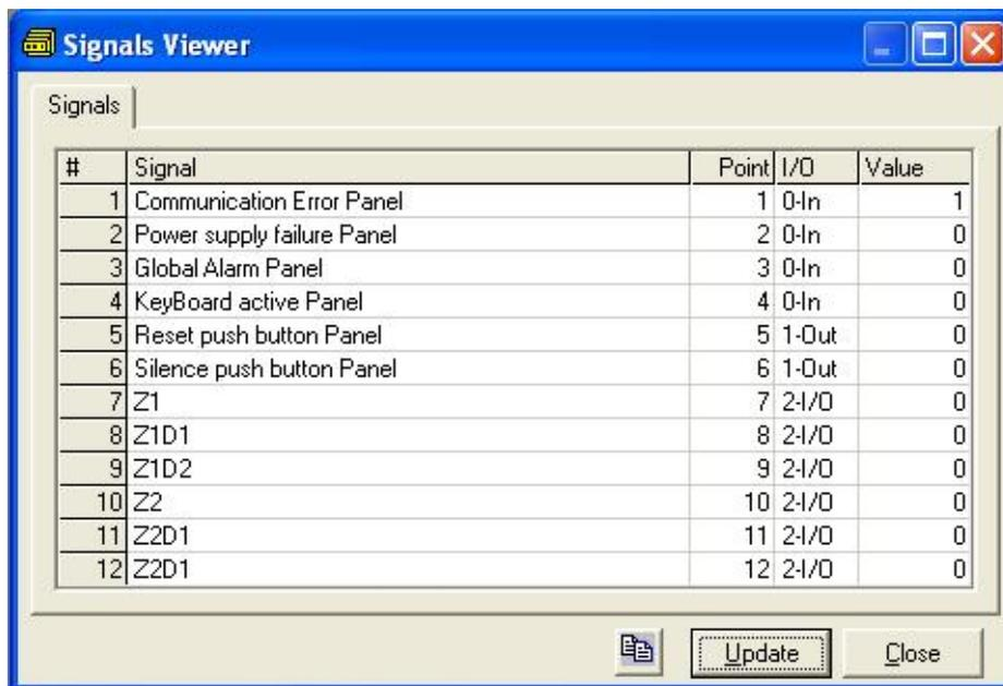
The signals viewer can be used although only one system is connected to the IBOX-MBS-ESSER, *ESSER* or *Modbus*, and is very useful for supervision and test.
