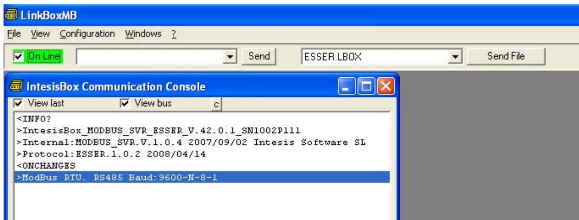
8. Modify the configuration as desired, save it and download the configuration file to IBOX-MBS-ESSER as explained before.
