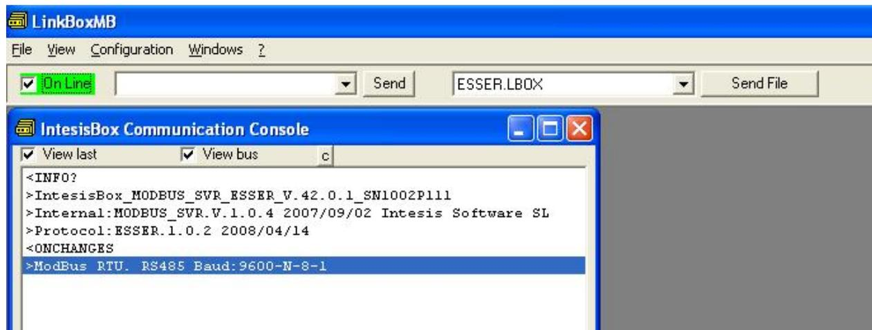
Once connected to IBOX-MBS-ESSER, all the options of LinkBoxMB are fully operative.
