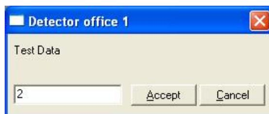
This tool is very useful to test the communication in the Modbus side from the Modbus master device for example, without the need to have the *ESSER* panel connected and running.
